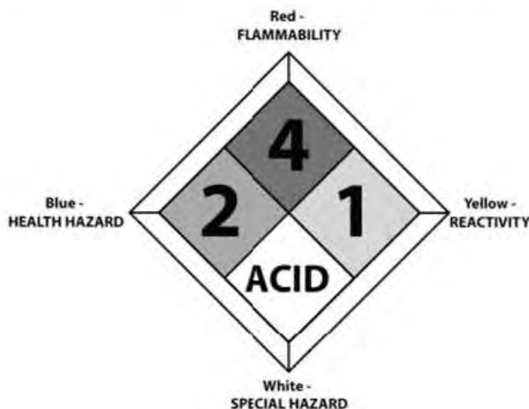
FIGURE 9.1 The NFPA 704 chemical hazard label. Each quadrant is labeled with its respective color and hazard.
