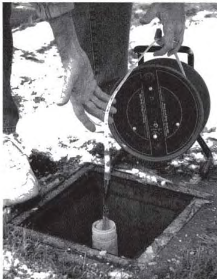
FIGURE 8.5 Electric probe used to measure water levels in monitoring wells.
