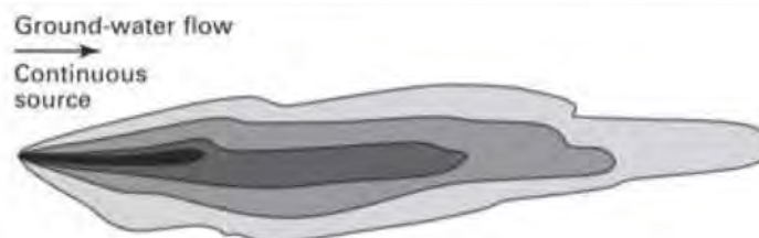
FIGURE 2.17 Plume resulting from the continuous injection of a tracer into a two-dimensional flow field. (Source: C. W. Fetter, 1994. Applied Hydrogeology, Third Edition . Upper Saddle River, New Jersey: Prentice-Hall, Inc.)
